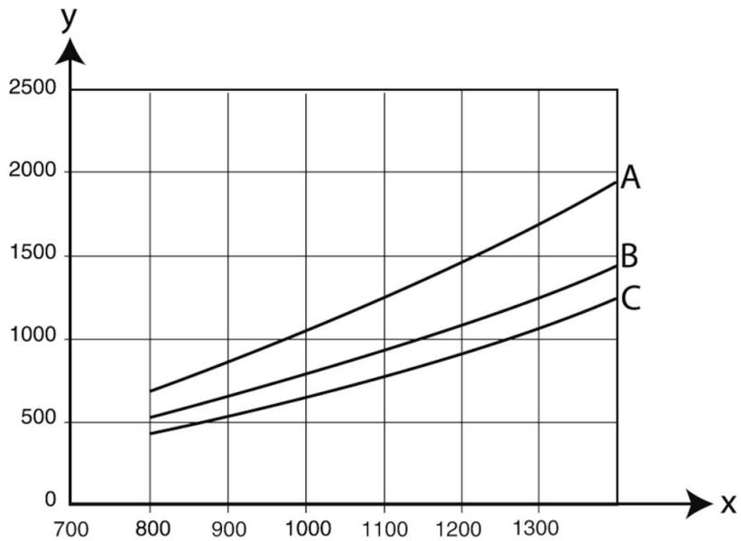
X: airflow, m<sup>3</sup>/h, Y: static pressure Pa,
