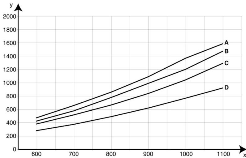
X: airflow m³/h, Y: static pressure Pa, A = 4 m horizontal, B =
